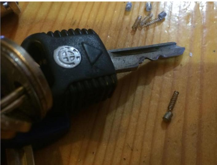
With the barrel out push the key you want to use in and observe which pins are proud:
