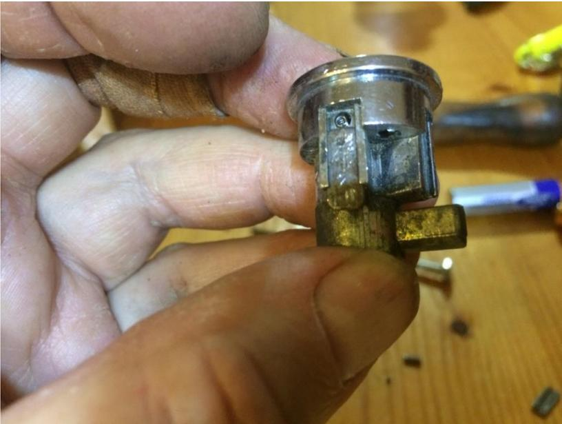
Use a sharp punch to tap them forward far enough to get a grip with pliers then keep your thumb over it so the tiny springs don't fly as you ease the plate out:
