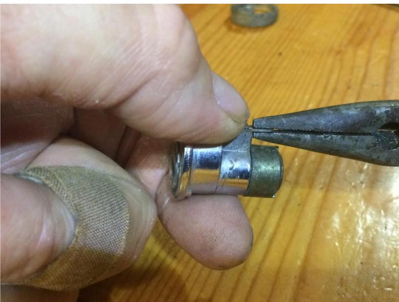
**Step 3** ....drill out the roll pin retaining the tongue: (1.5 mm drill bit)
