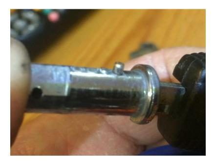
Note, in case they fall out, the pins in the barrel are pointed on the key side and flat on the side photographed. The flat face mates to the short pins pictured above.
