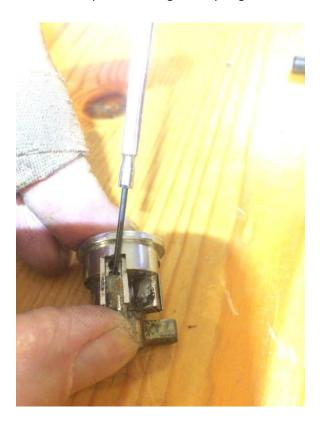
Reassembly of the rest is a straightforward matter. The roll pin may be reused if you were lucky with the drill otherwise a suitable small screw will replace it.
