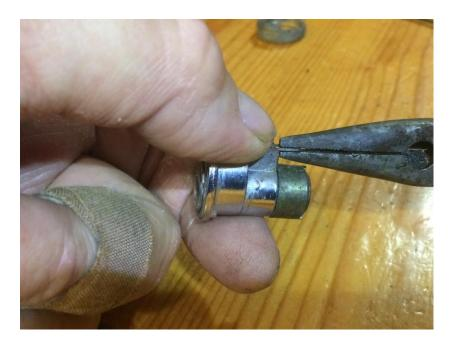
**Step 3** ....drill out the roll pin retaining the tongue: (1.5 mm drill bit)
