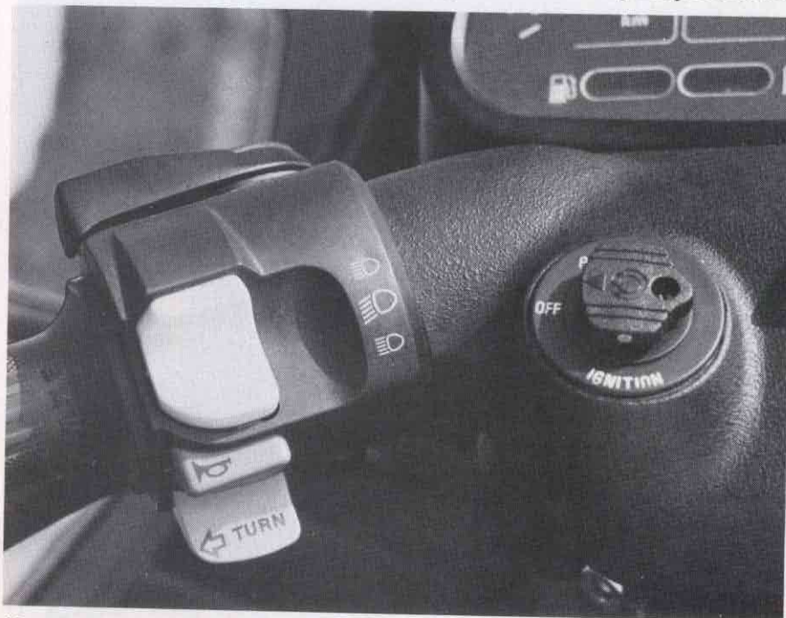
New Generation Strange Switches: Push for left turn, lift to honk! Headlight switch probably will be omitted on U.S. models. Choke level on top is the same as current BMW's.
