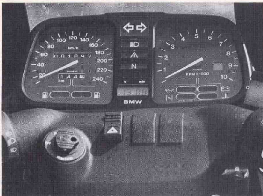
Warning lights abound but instrumentation remains easy to read at a glance. Note hazard flasher switch on padded dash; extra space is provided for two accessory switches.
