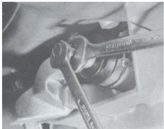
Clutch operating lever adjuster is used to set release mechanism
