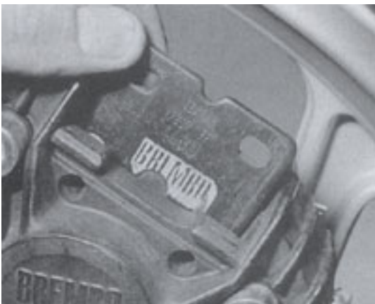
Remove pads, noting which way round each is fitted - check for uneven wear
