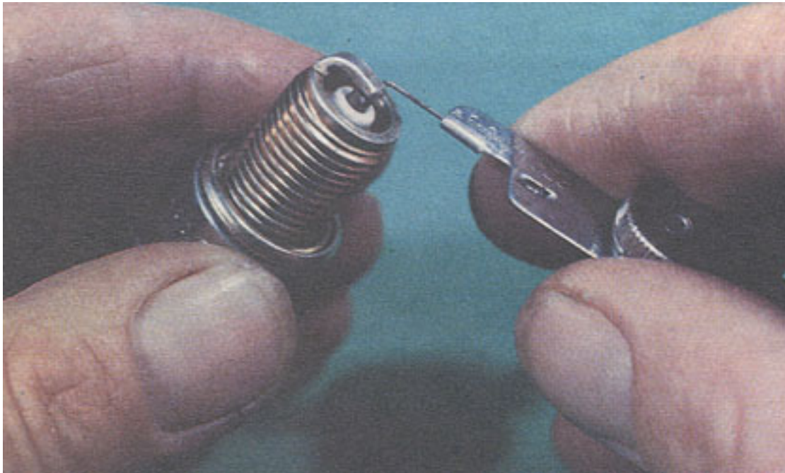
Checking plug gap with feeler gauges
