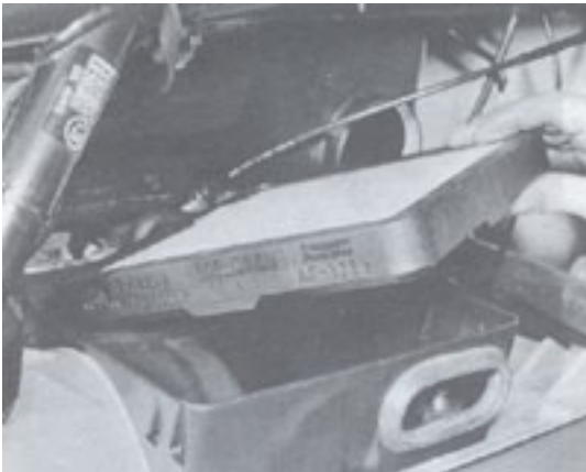
Ensure air filter element is correctly refitted to prevent entry of dirt into engine
