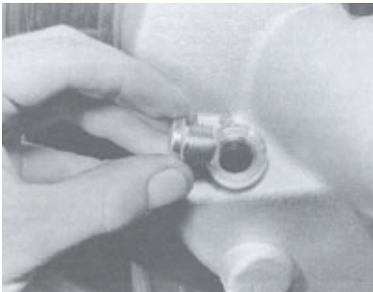
Remove final drive case filler plug to check oil level
