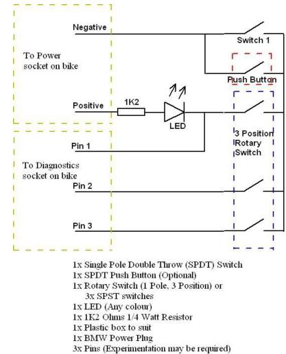
Sugar (OZ Brick rider) has published the schematic to build a cheap and easy 'BMW Test Box'. Here is its schematic:
