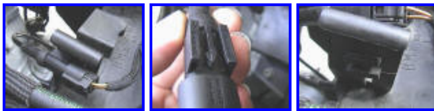
Connection at Motronic:
